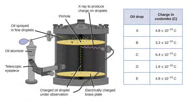
**Figure 2.7** Millikan's experiment measured the charge of individual oil drops. The tabulated data are examples of a few possible values.
