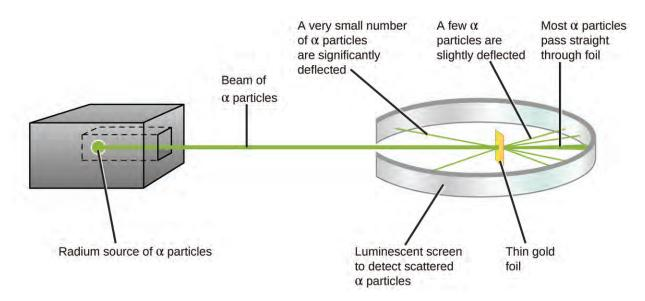
**Figure 2.9** Geiger and Rutherford fired  $\alpha$  particles at a piece of gold foil and detected where those particles went, as shown in this schematic diagram of their experiment. Most of the particles passed straight through the foil, but a few were deflected slightly and a very small number were significantly deflected.
