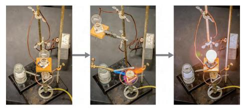
Figure 2.30 Sodium chloride melts at 801 °C and conducts electricity when molten. (credit: modification of work by Mark Blaser and Matt Evans)
