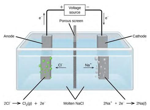
**Figure 17.19** Passing an electric current through molten sodium chloride decomposes the material into sodium metal and chlorine gas. Care must be taken to keep the products separated to prevent the spontaneous formation of sodium chloride.
