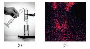
Figure 21.25 (a) The first Tc-99m generator (circa 1958) is used to separate Tc-99 from Mo-99. The  ${\rm MoO_4}^{2-}$  is retained by the matrix in the column, whereas the  ${\rm TcO_4}^-$  passes through and is collected. (b) Tc-99 was used in this scan of the neck of a patient with Grave's disease. The scan shows the location of high concentrations of Tc-99. (credit a: modification of work by the Department of Energy; credit b: modification of work by "MBq"/Wikimedia Commons)
