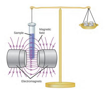
Figure 8.27 A Gouy balance compares the mass of a sample in the presence of a magnetic field with the mass with the electromagnet turned off to determine the number of unpaired electrons in a sample.
