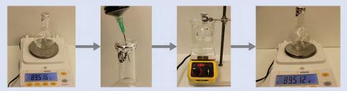
Figure 9.19 When the volatile liquid in the flask is heated past its boiling point, it becomes gas and drives air out of the flask. At  $t_{l \longrightarrow g}$ , the flask is filled with volatile liquid gas at the same pressure as the
