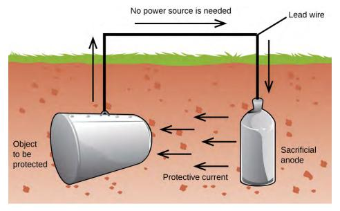
**Figure 17.18** One way to protect an underground iron storage tank is through cathodic protection. Using an active metal like zinc or magnesium for the anode effectively makes the storage tank the cathode, preventing it from corroding (oxidizing).
