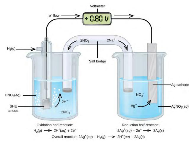
**Figure 17.8** A galvanic cell can be used to determine the standard reduction potential of Ag<sup>+</sup>. The SHE on the left is the anode and assigned a standard reduction potential of zero.
