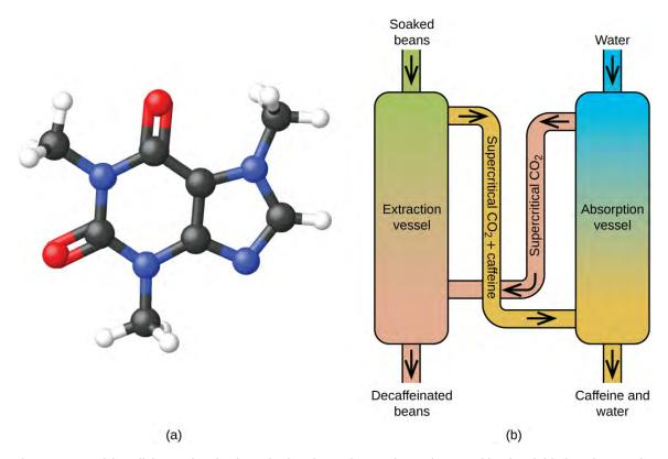
**Figure 10.36** (a) Caffeine molecules have both polar and nonpolar regions, making it soluble in solvents of varying polarities. (b) The schematic shows a typical decaffeination process involving supercritical carbon dioxide.
