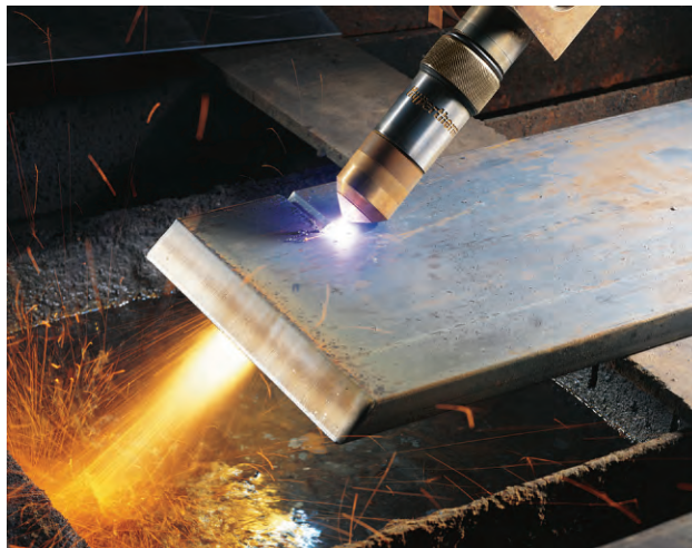
Figure 1.7 A plasma torch can be used to cut metal. (credit: “Hypertherm”/Wikimedia Commons)
