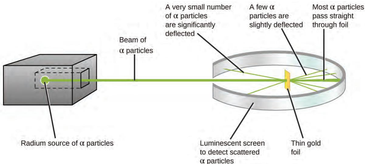
**Figure 2.9** Geiger and Rutherford fired  $\alpha$  particles at a piece of gold foil and detected where those particles went, as shown in this schematic diagram of their experiment. Most of the particles passed straight through the foil, but a few were deflected slightly and a very small number were significantly deflected.
