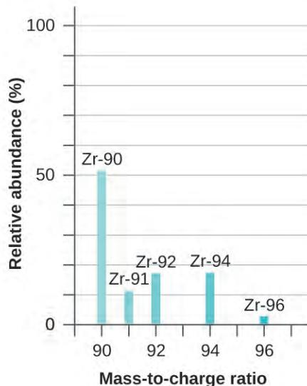
**Figure 2.15** Analysis of zirconium in a mass spectrometer produces a mass spectrum with peaks showing the different isotopes of Zr.
