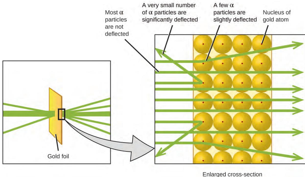
**Figure 2.10** The  $\alpha$  particles are deflected only when they collide with or pass close to the much heavier, positively charged gold nucleus. Because the nucleus is very small compared to the size of an atom, very few  $\alpha$  particles are deflected. Most pass through the relatively large region occupied by electrons, which are too light to deflect the rapidly moving particles.
