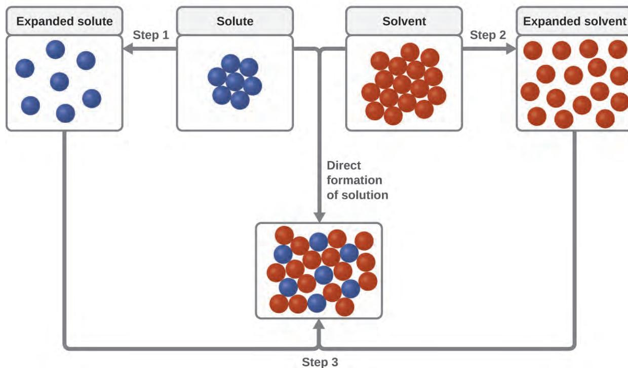
**Figure 11.4** This schematic representation of dissolution shows a stepwise process involving the endothermic separation of solute and solvent species (Steps 1 and 2) and exothermic solvation (Step 3).
