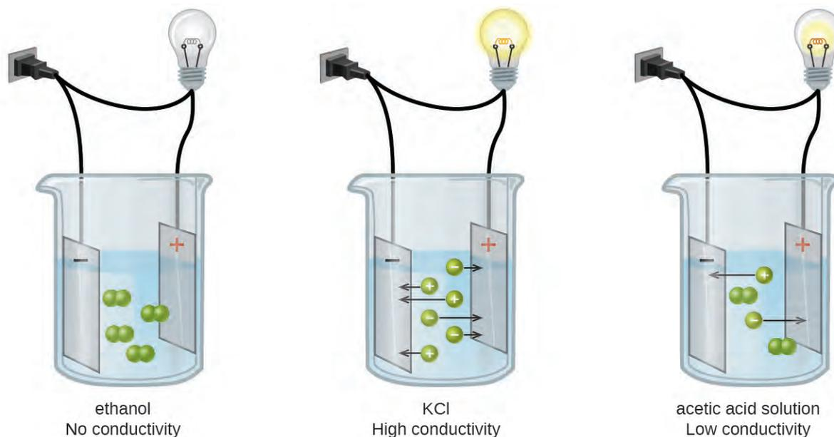
**Figure 11.7** Solutions of nonelectrolytes such as ethanol do not contain dissolved ions and cannot conduct electricity. Solutions of electrolytes contain ions that permit the passage of electricity. The conductivity of an electrolyte solution is related to the strength of the electrolyte.
