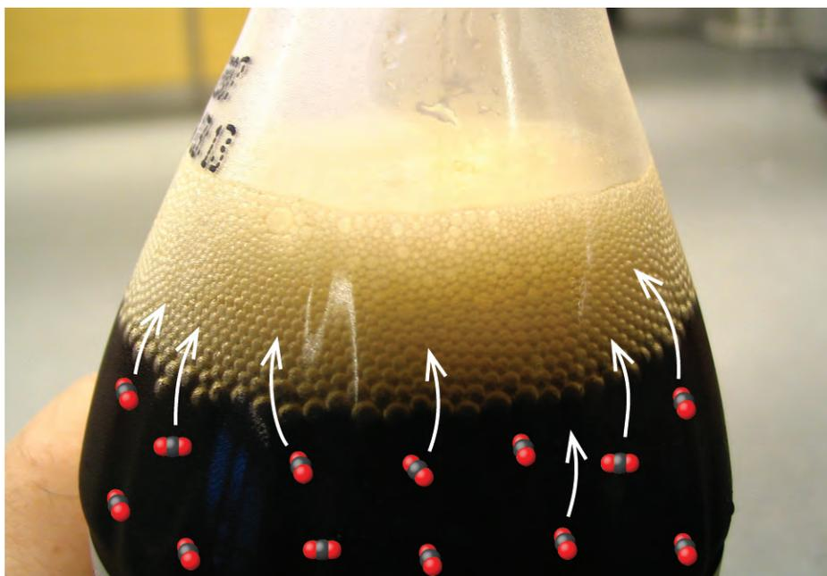
**Figure 11.11** Opening the bottle of carbonated beverage reduces the pressure of the *gaseous* carbon dioxide above the beverage. The solubility of CO<sub>2</sub> is thus lowered, and some *dissolved* carbon dioxide may be seen leaving the solution as small gas bubbles. (credit: modification of work by Derrick Coetzee)
