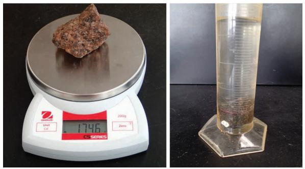
Figure 4.4 | Method to find the density of a rock. First the weight is measured on a digital scale and then the fluid displacement method is used to determine the volume. Author: Bradley Deline Source: Original Work License: CC BY-SA 3.0
