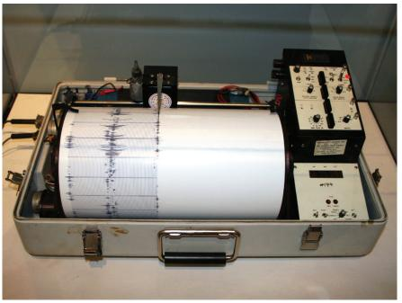
Figure 13.5 | A seismograph and the seismogram it produces. Author: User "Yamaguchi" Source: Wikimedia Commons License: CC BY-SA 3.0
