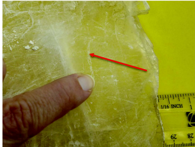
Figure 7.7 | An example of a scratch made by a fingernail on the mineral gypsum. The red arrow is pointing to the scratch. Gypsum, therefore, is softer than a fingernail.
